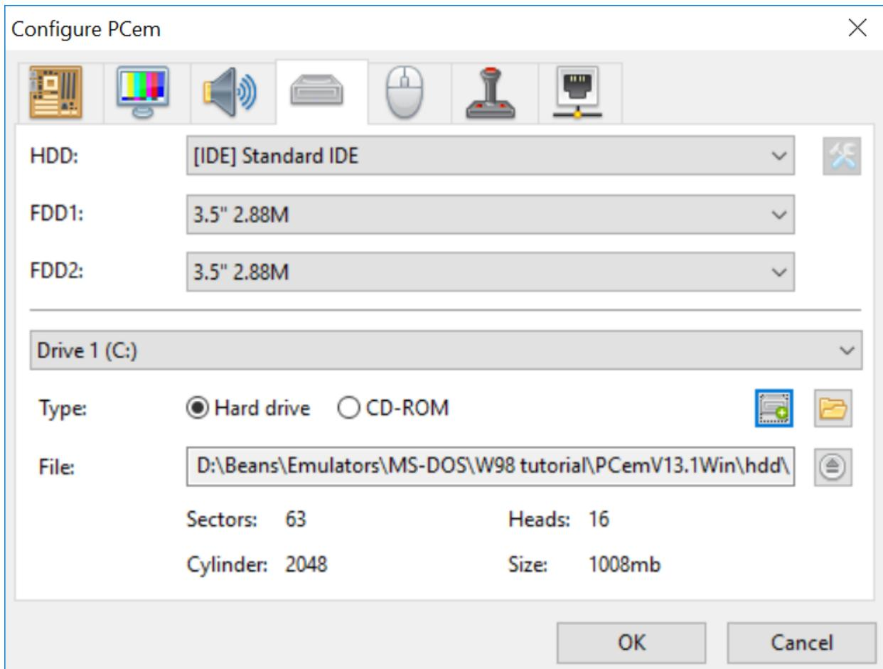
Set Drive C: as the main HDD, Drive D: as CD-ROM. Now create a new Hard drive image for Drive C: and set the parameters as the picture shows.
